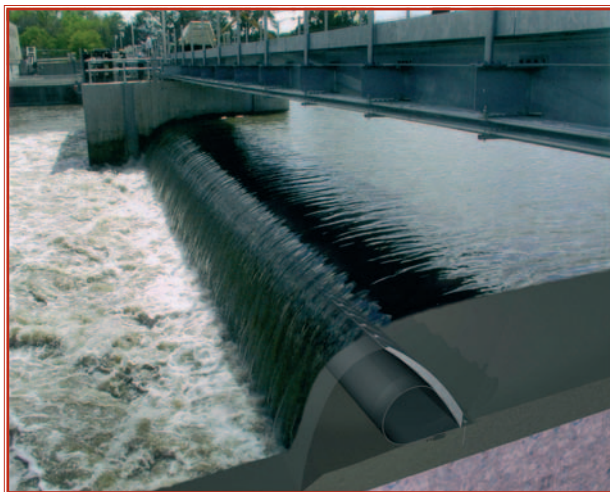
◀ Cross section through an Obermeyer spillway gate.
