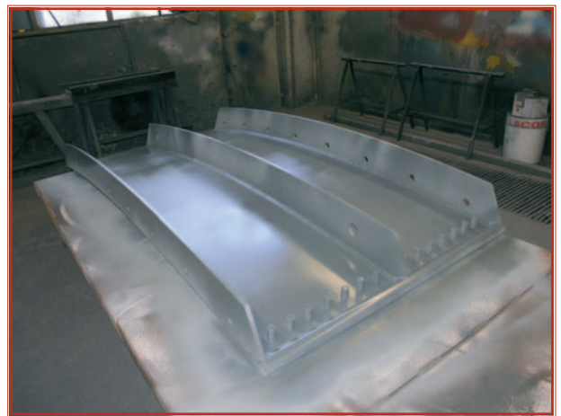
Ⓐ Fabrication and painting of gate panel in Europe.
